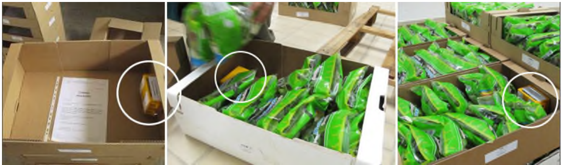
Figure 6 Data temperature recorder arranged into each packaging
