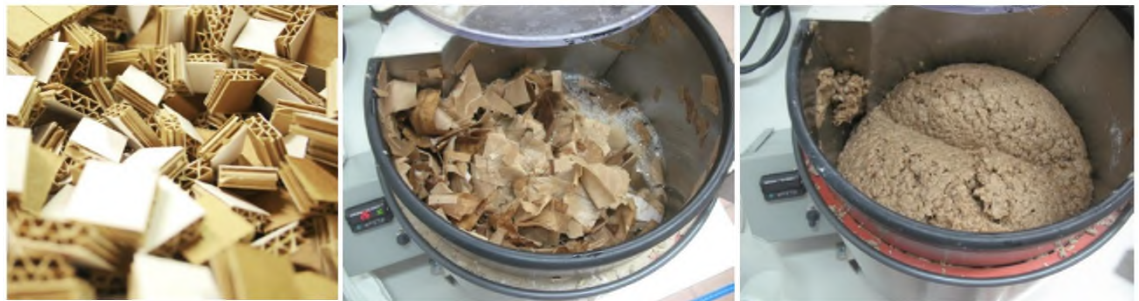
Figure 4 Realization of cellulose pulp into the pulper, starting from cardboard scraps
